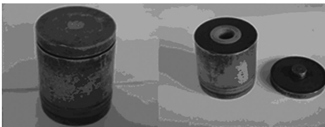
Figure 1. The measuring equipment of the composites in volume resistivity.
